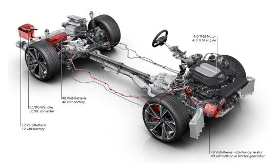
When the driver steps on the accelerator, the belt alternator starter will start the engine again. MHEV technology allows for start/stop operation at a speed of up to 22 km/h (*13.7 mph*). In everyday driving, it is possible to achieve fuel savings of up to 0.8 liters per 100 kilometers.
