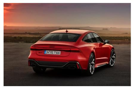
The rear end's sweeping spoiler lip and strip of lights linking the main rear lights together are among the characteristic defining features of the RS 7 Sportback\* and RS 7 Sportback performance\*. At a speed of 100 km/h (*62.1 mph*), a spoiler will extend from the tailgate. The RS exhaust system, with a large, chrome-colored oval tailpipe on each side, sits beneath an RS-specific bumper with a rear diffuser in gloss black.
