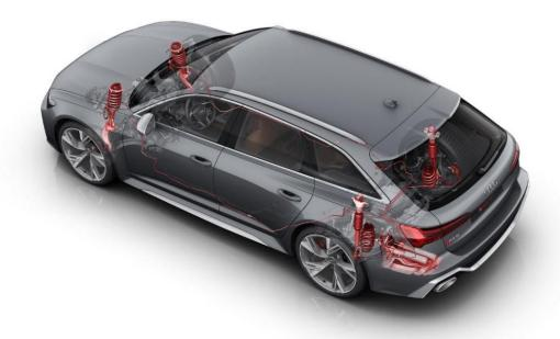
The generation of dampers with integrated valve has a more compact, lighter design and reduces pitch and rolling movements even more effectively. In addition, it enables the damping forces to be spread even more widely between the comfort, auto, and dynamic modes as well as more precise suspension adjustment for high damping forces, which occur during cornering at speed.
