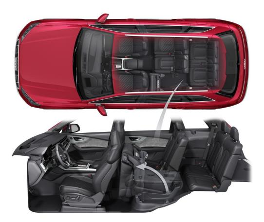
An electric tailgate is standard; foot-activated gesture control is available as an option. The electric luggage compartment cover is another convenience option. In addition, Audi optionally supplies the rear seat bench plus; all three seats can be moved individually fore/aft, and the backrest angle can be adjusted. There is also a third seat row with two seats that can be lowered electrically.
