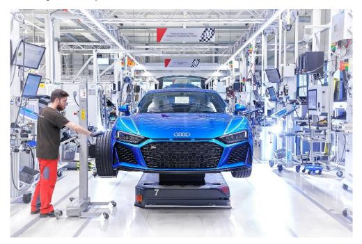
The finished body is transferred to the assembly area on a self-propelled assembly skid, which is known as a driverless transport system (DTS). The DTS utilizes high-power storage capacitors as its energy storage medium, and uses a laser scanner and RFID (Radio Frequency Identification) chips to navigate through the production floor areas. In the assembly area, which is laid out as a U-shaped chain, employees perform a large share of the work done by hand in 15 cycles.
