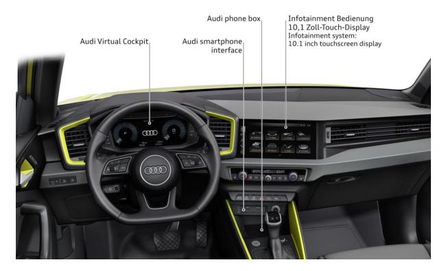
The new Audi A1 Sportback is fit for the digital future. Even the basic version comes standard with a fully digital instrument cluster with a high-resolution, 10.25-inch display. Also available as standard is a multi-function steering wheel in a sporty three-spoke design. It is available in different versions—round or flattened at the bottom, with or without rocker switches.
