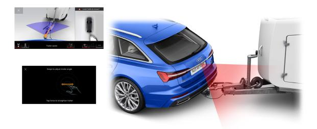
Behind the assist systems in the new Audi A6 Avant is a broad portfolio of sensors that are configured redundantly for maximum system reliability. Fully equipped, the set includes 24 sensors:
