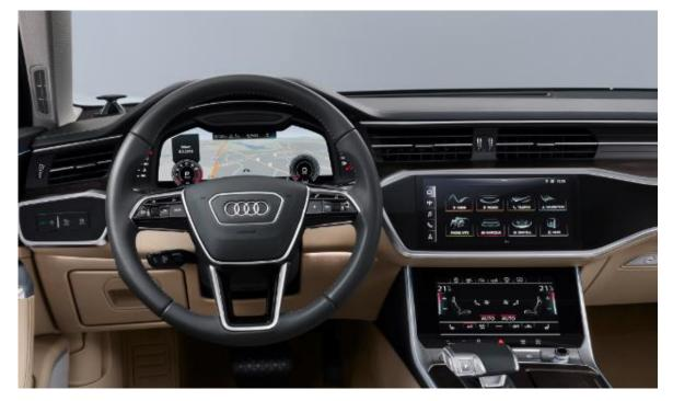
For other frequently used functions, the driver can also create shortcuts in the bottom screen and access various vehicle functions directly. These include radio stations, contacts from the phone book or apps.
