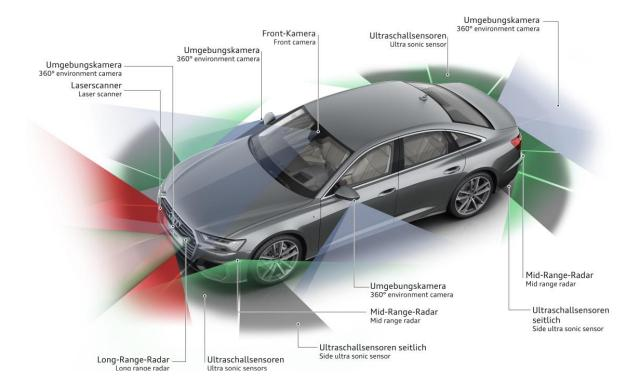
Fully equipped, the set includes 24 sensors:
