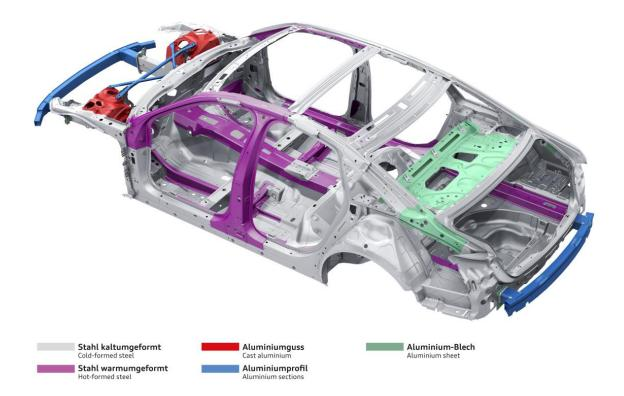
The body has been further developed in many aspects: The newly designed structural front end and the torsion rings contribute substantially to the high body rigidity. The front axle is joined more rigidly than on the predecessor model. The optimized load application points and the meticulous tuning of the resonances improve the body's acoustic characteristics. In the exhaust system, the silencers are connected to each other in a unique way to minimize lowfrequency noise.
