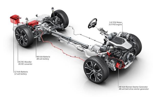
The Audi A7 Sportback is equipped standard with the new <u>mild-hybrid technology</u> (MHEV, mild hybrid electric vehicle) for greater efficiency and comfort. The technology reduces consumption by as much as 0.7 liters of fuel per 100 kilometers in real driving. With the 3.0 TFSI and 3.0 TDI, it is based on a newly developed 48-volt primary electrical system. It comprises a compact lithium-ion battery and a belt alternator starter (BAS) that is connected to the crank shaft.
