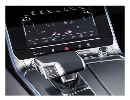
The new Audi A7 Sportback uses MMI touch response, the fully digital operating concept from the flagship A8 that can be operated as intuitively as a smartphone with touch and swipe gestures. Two touch displays with haptic and acoustic feedback replace the rotary pushbutton and many buttons from the previous model. They transport Audi's quality standards into the digital age and offer a high degree of operating safety.
